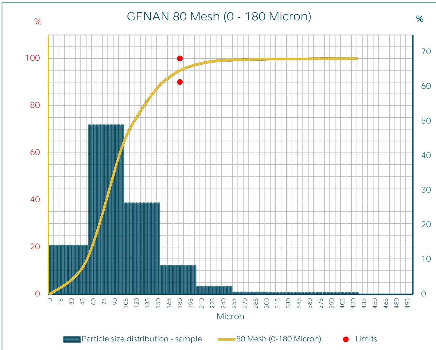
An Air Jet Sieve from Hosokawa Alpine is used to make a sieve analysis of the material / Test sieving in compliance with DIN ISO 3101-1.
